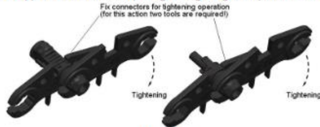
Figure 14 Tightening the connectors with Opening tool
