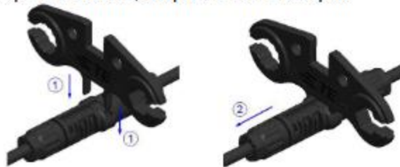
Figure 13 Disconnect the connectors
